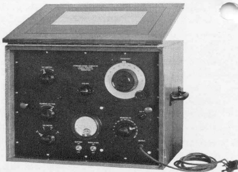
A simultaneous development for servicing and testing over a wide frequency range, the TYPE 601-A Standard-Signal Generator of July, 1931
