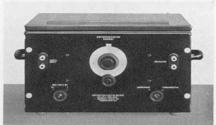
The TYPE 536 Distortion-Factor Meter measures the 400-cycle distortion in an audio-frequency system
