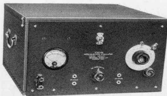
TYPE 375 Station Piezo-Electric Oscillator, the broadcast-station frequency monitor of 1926
