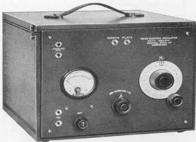
The early TYPE 275 Piezo-Electric Oscillator made no provision for temperature control of the Quartz Plate
